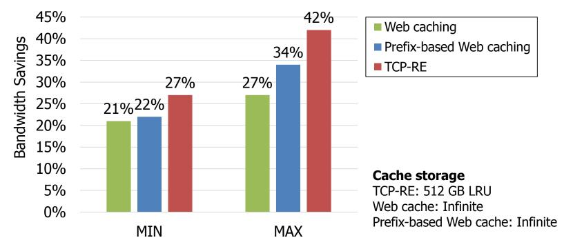
TCP-RE outperforms even with the smaller cache size than Web caching.
