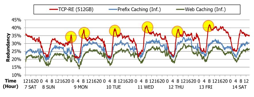
TCP-RE can detect the peak redundancy.
