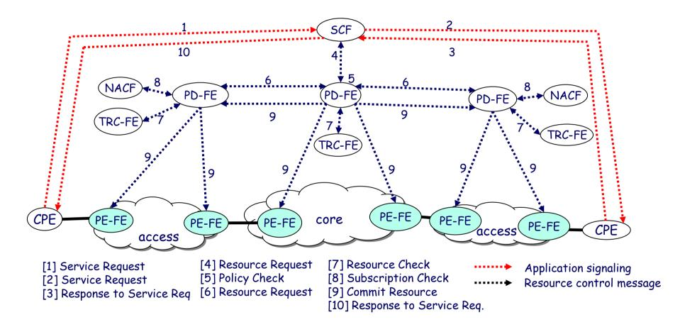
■ Flow based control at the edge of the network
